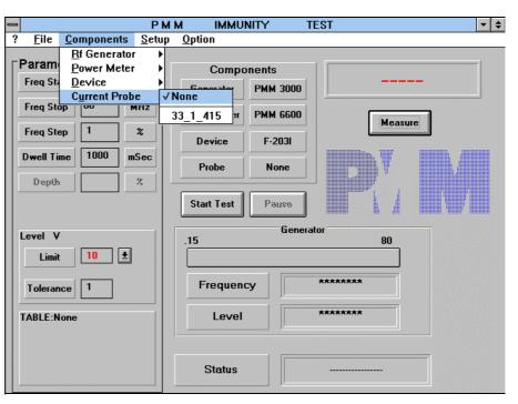
Selecting the Probe model will take into account the correction factors of the probe during the measurement via the power meter, in order to give the right reading of the current flowing in the cables of the EUT.
