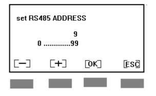
Use key [-] or [+] to increase or decrease the address. Push OK to confirm. Push ESC to exit ADDRESS mode of operation.
