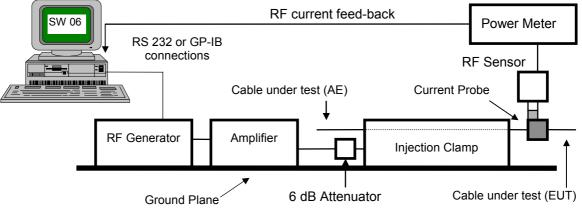
Fig. 6-1 Block Diagram of Test Setup with Injection Clamp
