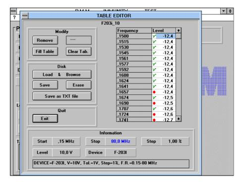
You can also save this new table and use it for the debugging phase, in order to half reduce the time of the complete procedure, but in this case you will need to load this modified table from the Setup menu and select **None** as Current Probe in the Components menu.
