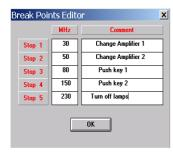
All that is needed is to insert the stop frequencies in the **MHz** column, add an eventual comment on the same line and close the window by clicking on the "**OK**" button.
